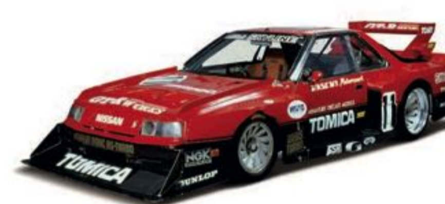
1983 Skyline Super Silhouette (KDR30) Engine L220B (4-cyl. in line, DOHC), 2,082cc Maximum power Over 419kW (570PS)/7,600rpm Maximum Torque Over 539Nm (55kgm)/6,400rpm
