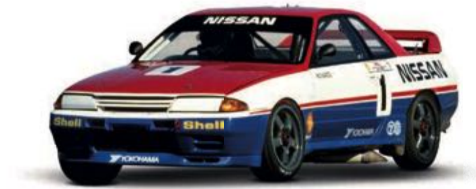
1991 Skyline GT-R (BNR32) Engine RB26DET (6-cyl. in line, DOHC), 2,568cc Maximum power Over 297kW (400PS)/7,200rpm Maximum Torque Over 441Nm (45.0kgm)/4,800rpm
