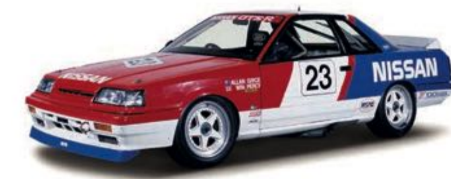
1988 Skyline GTS-R (KHR31) Engine RB20DET-R (6-cyl. in line, DOHC), 2,028cc Maximum power 294kW (400PS)/7,200rpm Maximum Torque 412Nm (42.0kgm)/6,000rpm
