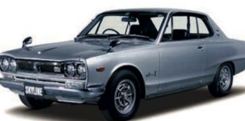
1972 Skyline H/T 2000 GT-X (KGC10) Engine L20T (6-cyl. in line, OHC), 1,998cc Maximum power 98kW (130PS)/6,000rpm Maximum Torque 172Nm (17.5kgm)/4,400rpm
