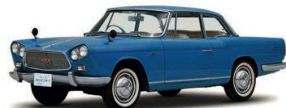
1962 Skyline Sports (BLRA-3) Engine GB4 (4-cyl. in line, OHV), 1,862cc Maximum power 69kW (94PS)/4,800rpm Maximum Torque 153Nm (15.6kgm)/3,600rpm
