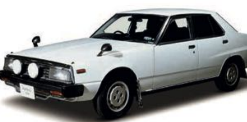
1980 Skyline 2000GT (HGC211) Engine L20 (6-cyl. in line, OHC), 1,998cc Maximum power 85kW (115PS)/6,800rpm Maximum Torque 162Nm (16.5kgm)/3,600rpm
