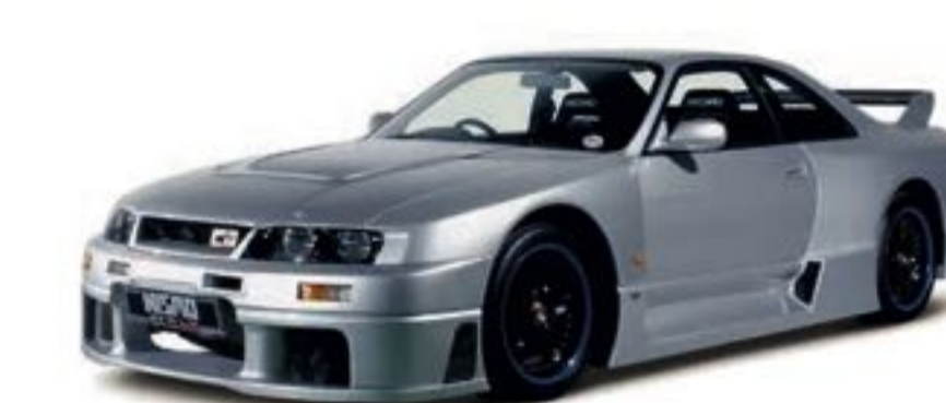
1996 Skyline GT-R (BCNR33) Engine RB26DET (6-cyl. in line, DOHC), 2,568cc Maximum power 224kW (305PS)/6,500rpm Maximum Torque 373Nm (38.0kgm)/4,500rpm
