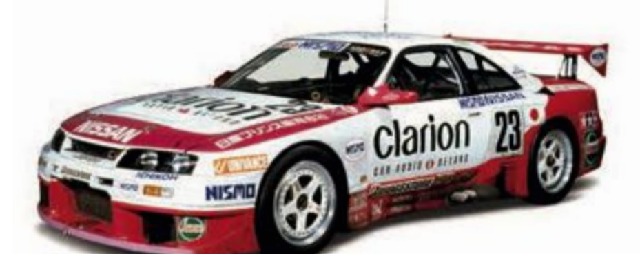
1996 Skyline GT-R (BCNR33) Engine RB26DET (6-cyl. in line, DOHC), 2,795cc Maximum power Over 441kW (600PS)/7,000rpm Maximum Torque Over 618Nm (63.0kgm)/5,500rpm
