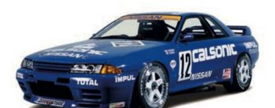
1993 Skyline GT-R (BNR32) Engine RB26DET (6-cyl. in line, DOHC), 2,568cc Maximum power 405kW (550PS)/7,600rpm Maximum Torque 490Nm (50kgm)/6,000rpm
