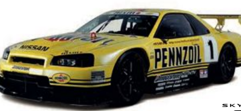
1999 Skyline GT-R (BNR34) Engine RB26DET (6-cyl. in line, DOHC), 2,708cc Maximum power 368kW (500PS)/6,000rpm Maximum Torque Over 708Nm (72.0kgm)/4,400rpm
