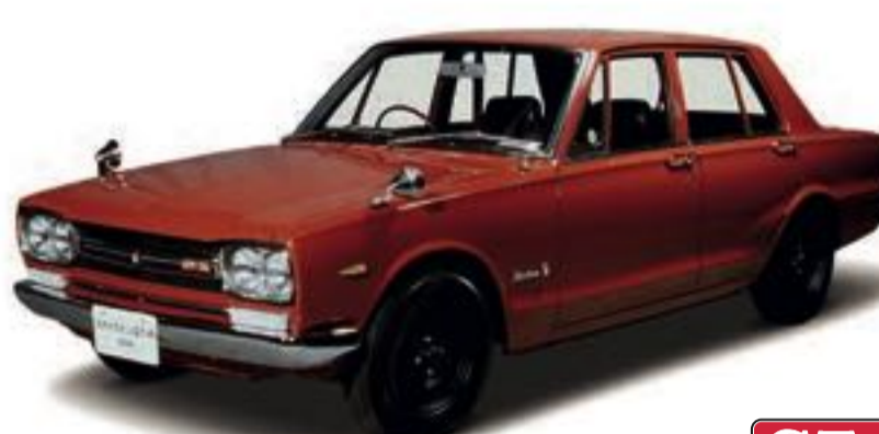
1969 Skyline 2000GT-R (PGC10) Engine S20 (6-cyl. in line, DOHC), 1,989cc Maximum power 118kW (160PS)/7,000rpm Maximum Torque 177Nm (18.0kgm)/5,600rpm
