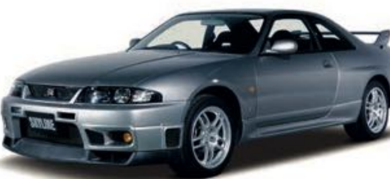
1997 Skyline GT-R V Specifications (BCNR33) Engine RB26DET (6-cyl. in line, DOHC), 2,568cc Maximum power 206kW (280PS)/6,800rpm Maximum Torque 358Nm (36.5kgm)/4,400rpm
