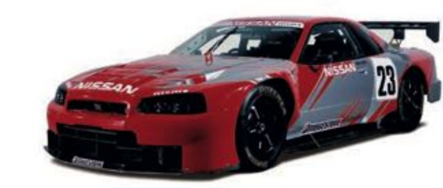
2002 Skyline GT-R (BNR34) Engine RB26DET (6-cyl. in line, DOHC), 2,708cc Maximum power 338kW (460PS)/6,000rpm Maximum Torque 686Nm (70kgm)/4,400rpm
