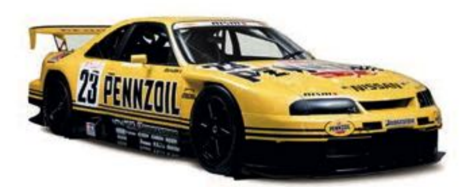
1998 Skyline GT-R (BCNR33) Engine RB26DET (6-cyl. in line, DOHC), 2,708cc Maximum power Over 368kW (500PS) Maximum Torque Over 708Nm (72.0kgm)
