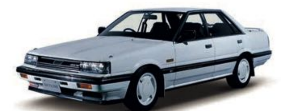
1986 Skyline GTS Twin-cam (KRR31) Engine RB20DET (6-cyl. in line, DOHC turbo), 1,998cc Maximum power 140kW (190PS)/6,400rpm Maximum Torque 240Nm (24.5kgm)/4,800rpm
