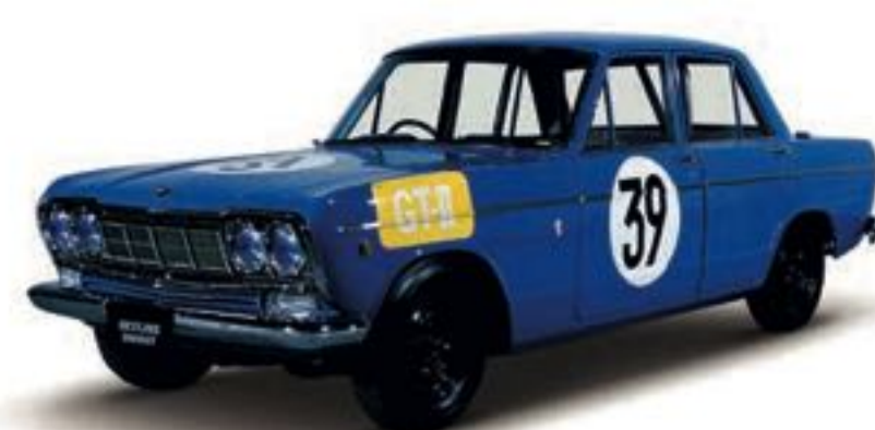
1964 Skyline 2000GT (S54) Engine G7 (6-cyl. in line, OHC) 1,988cc Maximum power 121kW (165PS)/6,800rpm Maximum Torque 180Nm (18.4kgm)/6,000rpm
