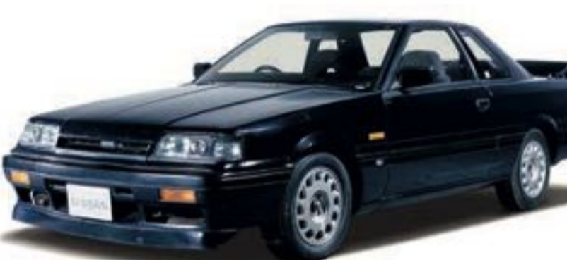
1987 Skyline 2000GTS-R (KHR31) Engine RB20DET-R (6-cyl. in line, DOHC), 1,998cc Maximum power 154kW (210PS)/6,400rpm Maximum Torque 245Nm (25kgm)/4,800rpm
