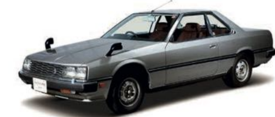
1981 Skyline H/T Turbo 2000GT-ES (KHR30) Engine L20ET (6-cyl. in line, OHC), 1,998cc Maximum power 107kW (145PS)/6,600rpm Maximum Torque 208Nm (21.0kgm)/3,200rpm
