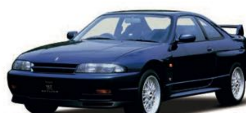
1993 Skyline GT-R (BCNR33) Engine RB26DET (6-cyl. in line, DOHC), 2,568cc Maximum power 206kW (280PS)/6,800rpm Maximum Torque 358Nm (36.5kgm)/4,400rpm
