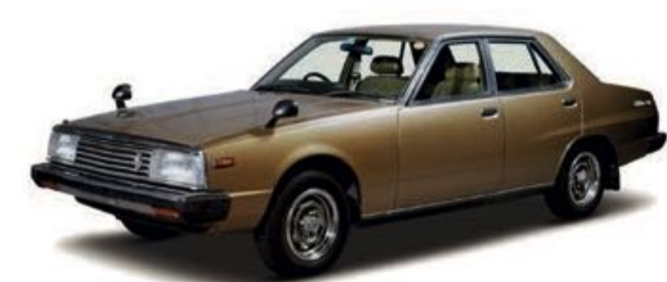
1980 Skyline 2000GT-EL (HGC211) Engine L20E (6-cyl. in line, OHC), 1,998cc Maximum power 92kW (125PS)/6,000rpm Maximum Torque 167Nm (17.0kgm)/4,000rpm
