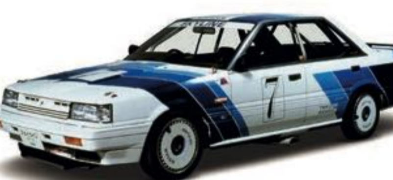
1985 Skyline GT Passage Twin-cam (KRR31) Engine RB20DET (6-cyl. in line, DOHC), 1,998cc Maximum power Over 221kW (300PS) Maximum Torque Over 343Nm (35.0kgm)
