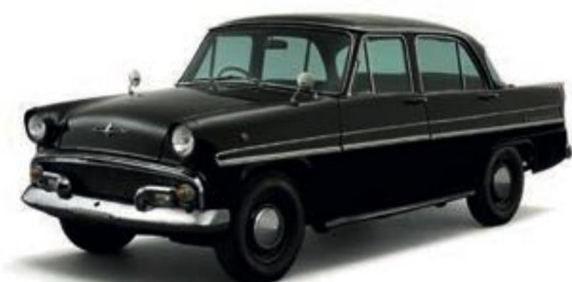
1957 Skyline Deluxe (ALSID-1) Engine GA30 (4-cyl. in line, OHV), 1,484cc Maximum power 44kW (60PS)/4,400rpm Maximum Torque 105Nm (110.7kgm)/3,200rpm
