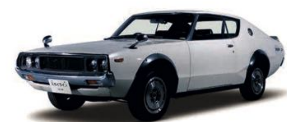
1973 Skyline H/T 2000GT-R (KPGC110) Engine S20 (6-cyl. in line, DOHC), 1,989cc Maximum power 118kW (160PS)/7,000rpm Maximum Torque 177Nm (18.0kgm)/5,600rpm
