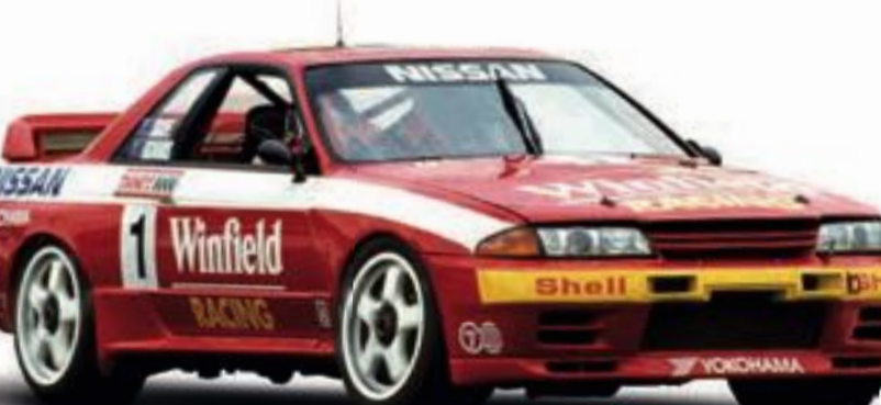
1992 Skyline GT-R (BNR32) Engine RB26DET (6-cyl. in line, DOHC), 2,568cc Maximum power Over 297kW (400PS)/7,200rpm Maximum Torque 441Nm (45kgm)/4,800rpm
