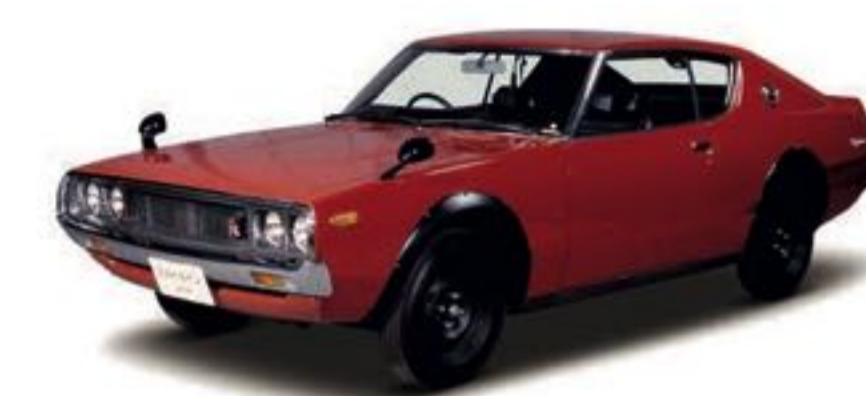
1973 Skyline H/T 2000GT-R (KPGC110) Engine S20 (6-cyl. in line, DOHC), 1,989cc Maximum power 118kW (160PS)/7,000rpm Maximum Torque 177Nm (18.0kgm)/5,600rpm
