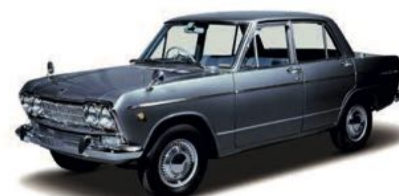
1965 Skyline 1500 Deluxe (S50) Engine G1 (4-cyl. in line, OHV), 1,484cc Maximum power 51kW (70PS)/4,800rpm Maximum Torque 113Nm (11.5kgm)/3,600rpm
