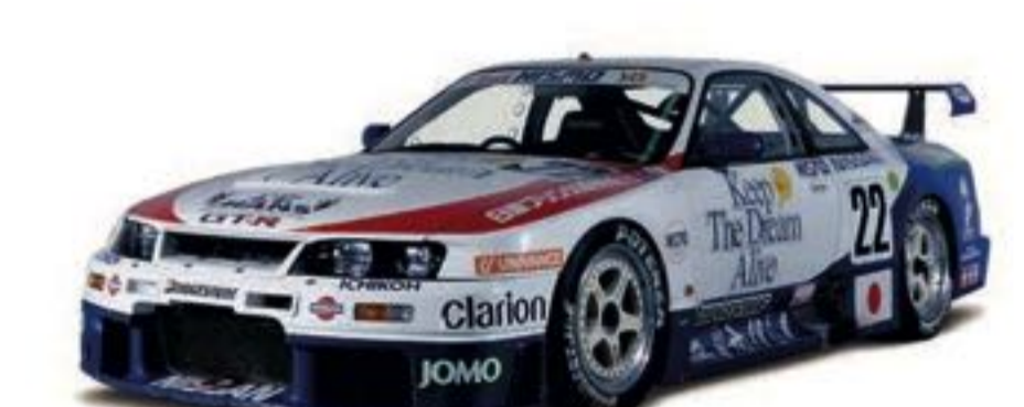
1995 Skyline GT-R (BCNR33) Engine RB26DET (6-cyl. in line, DOHC), 2,568cc Maximum power Over 297kW (400PS)/7,200rpm Maximum Torque Over 441Nm (45.0kgm)/4,800rpm
