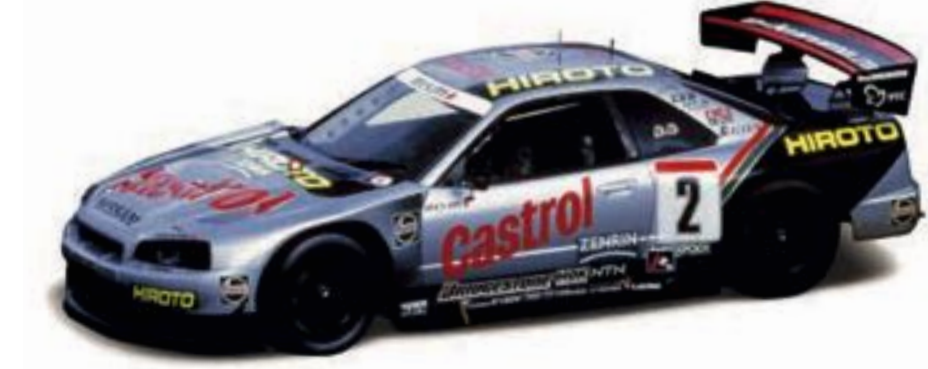
2000 Skyline GT-R (BNR34) Engine RB26DET (6-cyl. in line, DOHC), 2,708cc Maximum power Over 338kW (460PS)/6,000rpm Maximum Torque Over 686Nm (70kgm)/4,400rpm
