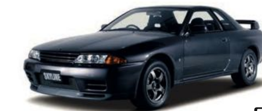
1989 Skyline GT-R (BNR32) Engine RB26DET (6-cyl. in line, DOHC), 2,568cc Maximum power 206kW (280PS)/6,800rpm Maximum Torque 353Nm (36kgm)/4,400rpm
