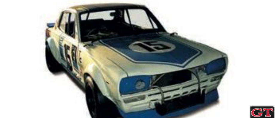
1972 Skyline H/T 2000GT-R (KPGC10) Engine S20 (6-cyl. in line, DOHC), 1,989cc Maximum power 184kW (250PS)/8,400rpm Maximum Torque 211Nm (21.5kgm)/6,800rpm
