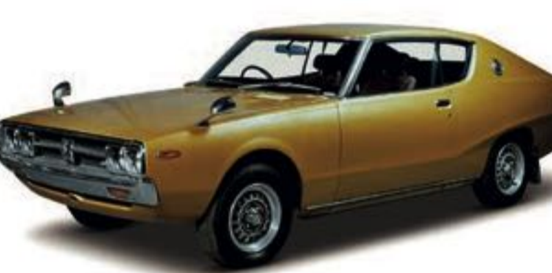
1976 Skyline H/T 2000GT-E/GTX-E (KGC111) Engine L20E (6-cyl. in line, OHC), 1,998cc Maximum power 96kW (130PS)/6,000rpm Maximum Torque 167Nm (17.0kgm)/4,000rpm
