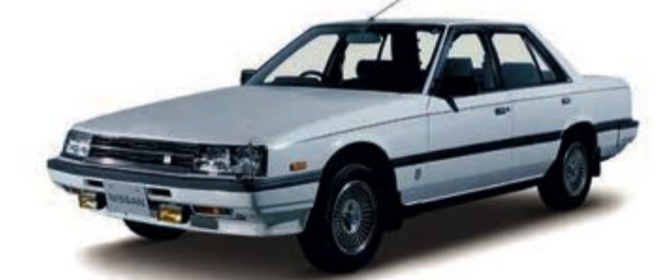
1983 Skyline 2000GT-E/X (HR30) Engine L20E (6-cyl. in line, OHC), 1,998cc Maximum power 92kW (125PS)/6,000rpm Maximum Torque 167Nm (17.0kgm)/4,400rpm
